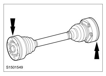
**NOTE:** The grooves on the circumference of the joints should be on the outside.
